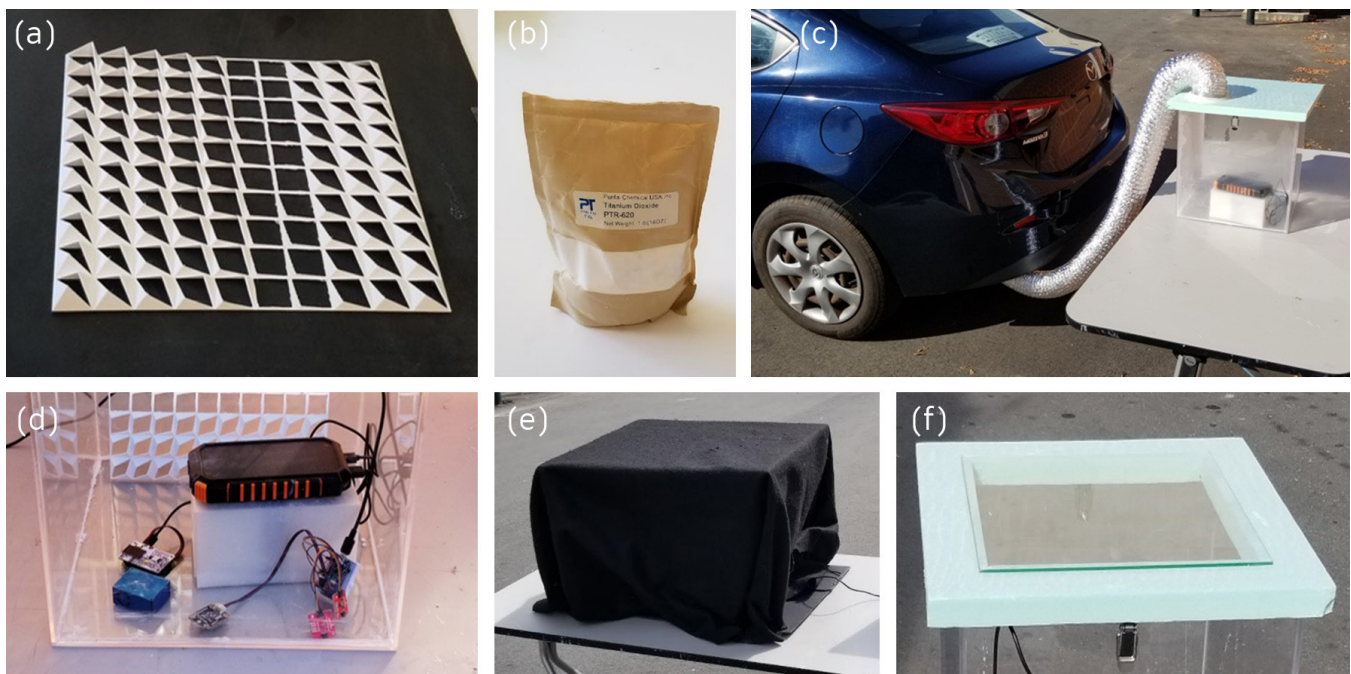
Figure 2 Experiment Setup. (a) Photocatalytic facade sample, (b) TiO 2 Powder, (c) Testing chamber and pollutant gases, (d) Sensors and data logger, (e) Black cloth for the control experiment, (f) Glass lid with rigid foam
